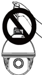
2. Don't pick up the cable by hand, it may cause connection problem with cable.
